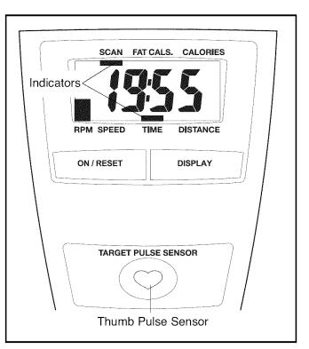
Speed—This display shows your pedaling speed, in miles or kilometers per hour.
